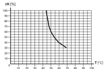
and under the curve may be selected. For instance at 60°C temperature you can set up to 40% rel. air humidity. In order to set a higher humidity you will need first to reduce the temperature.
