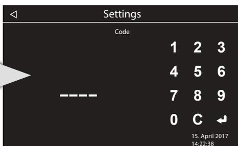
Give in the access code for the service level. Correction with „C“. Confirm entry with the „enter“ button.
