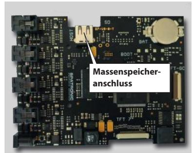
In the case of power supply loss the control panel will attempt to resume the update process. If the display panel does not start or shows a boot load error press firmly on the “reset” button on the board next to the battery cell. The unit will reboot and offer update options dialogue, allowing you to attempt to repeat the update.
