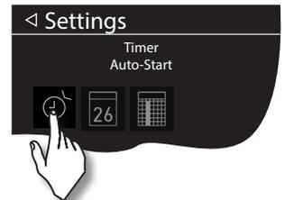
Notice that the programmed time means the real time, not the time delay. In order to cancel this program set the start time back to „-:-“ and confirm the setting.
