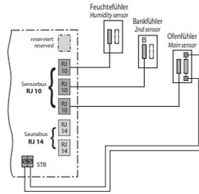
Connection overview for temperature sensor, bench sensor and humidity sensor.
