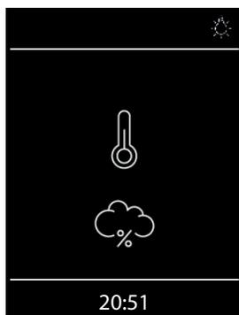
Display in standby mode by humid (Bi-O) sauna operation (Emotec H only).
