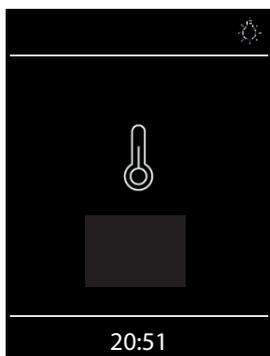
Display in standby mode by dry (Finnish) sauna operation (Emotec D and H).
