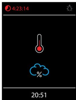
**When the sauna is switch on** - the thermometer symbol starts to pulse red during the heating up time, after this it will continuously light in red.
