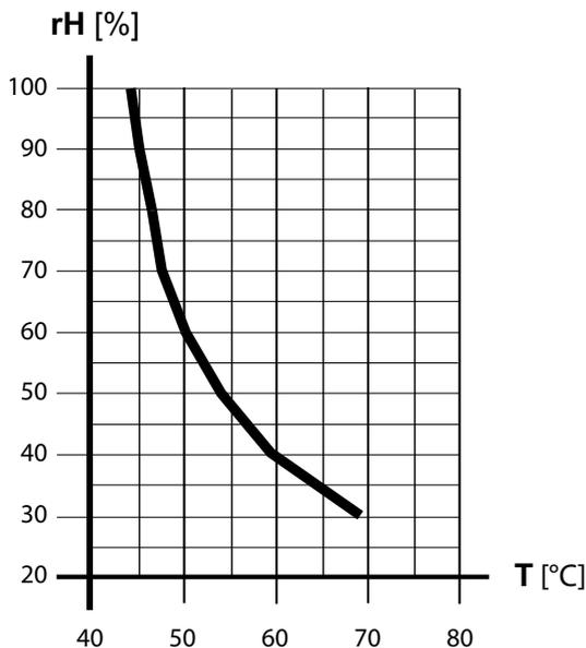
☒ Characteristics curve for temperature/humidity
