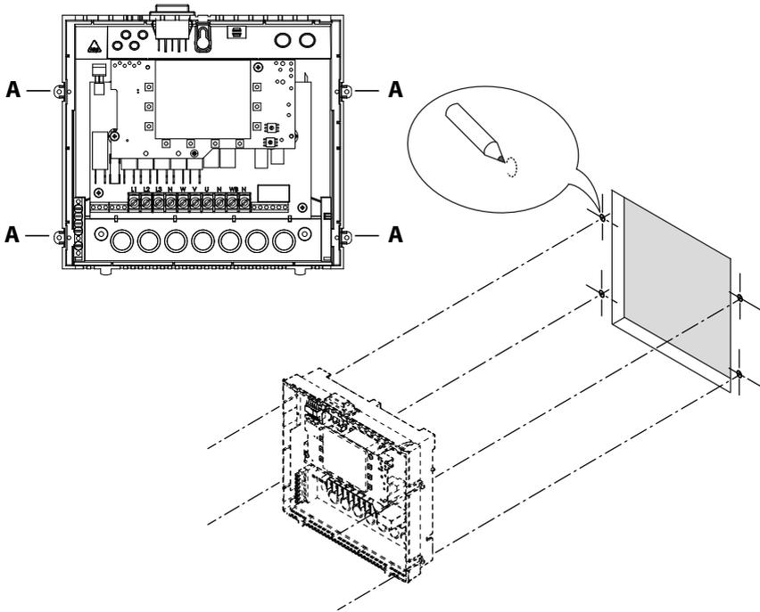
**A** Tabs with mounting holes for screws
