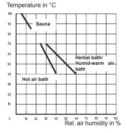
The humidity intensity shown in the display corresponds to the time proportional evaporator setting. Therefore, the relative air humidity is <u>not</u> preselected or shown on the display, but rather the switch-on frequency of the evaporator in percent. The graphic is intended to clarify this.
