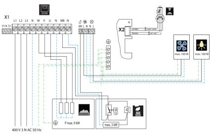
Warning: Always connect the neutral conductor of the sauna oven. During steam operation, one phase of the oven is shut down; therefore the heating load is no longer symmetrical. The result is that the neutral wire is no longer current-free.
