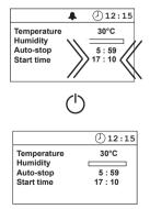
If the sauna unit is to be used without preselection time, --: -- must be entered in the display under preselection time.
