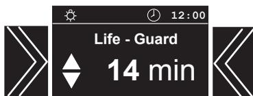
After expiration of the "Life - Guard" - time the sauna heater is switched off and the set "Life - Guard" - time blinks.
