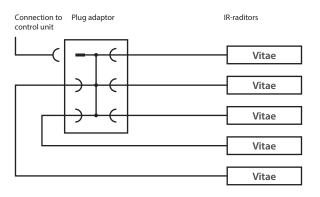
By 750 W radiators max. 4 units (3500W) possible by 16 A capable connection line.
