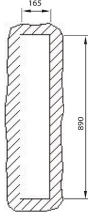
**Attention!** Make sure to provide sufficient air circulation behind and above the radiator. The space above the radiator must not be blocked, so that the warm air may rise freely. **Risk of fire!**
