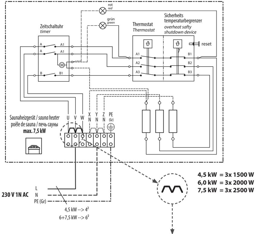
By 230V 1N connection the 3-pole copper bridge must be fitted on the U/V/W terminals. This bridge is included in the delivery scope.
